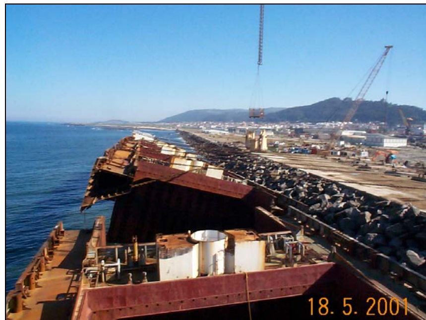
Figure 2: Parbuckle of forward section.
