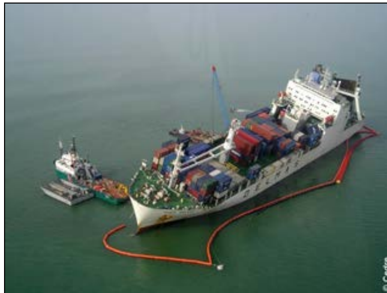
Figure 5: Removal of hydrocarbons.
